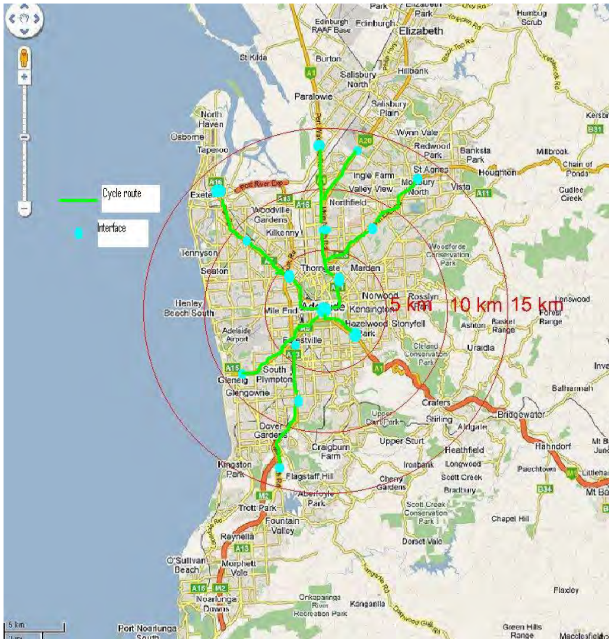
Figure 7.3 Typical system boundary with nodes or hubs marked along major arterial routes
