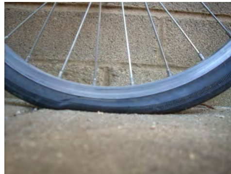
Figure 10.13 Tyre under low pressure, showing flattened bottom tread section
